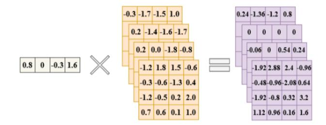
Features from non-imaging branch will emphasis or restrain the corresponding feature maps from imaging branch
